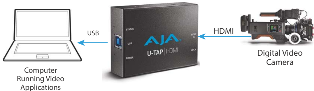
Figure 5. Typical U-TAP-HDMI Laptop System Connections
