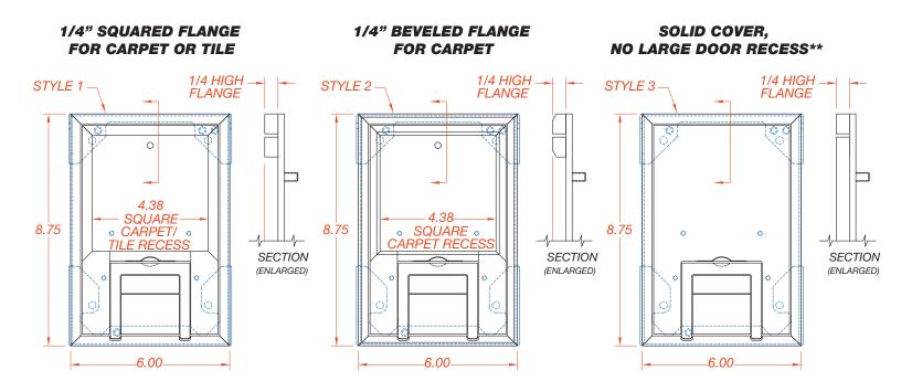
\*\*Note: Cover Shim Kit (FL-200-CSK) may be required to set the height of box "Pre-Pour" so the top of Finish Cover matches top of finished floor.
