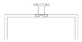
Attach the eBeam receiver to the bracket using the magnetic mounts on the bracket.
