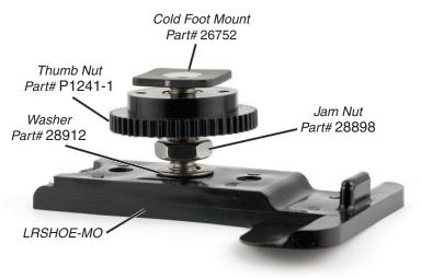
Assemble the parts as shown. The nut in the bracket is an elliptical tensioning type. A wrench is needed to insert the cold foot stud.
