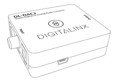
The DigitaLinx DL-DAC2 is a PCM two channel to stereo audio converter. The DL-DAC2 features optical and digital coaxial input audio connections. Analog output is simultaneously available on the 3.5mm jack and the stereo RCA jacks.
