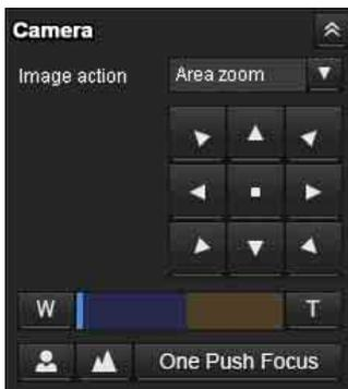
You can operate the pan/tilt, moving to the home position, zoom, and focus of the camera by using the control panel for the monitor image currently displayed (page 15).
