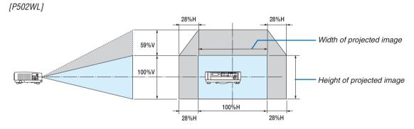
Description of symbols: V indicates vertical (height of the projected image), H indicates horizontal (width of the projected image).
