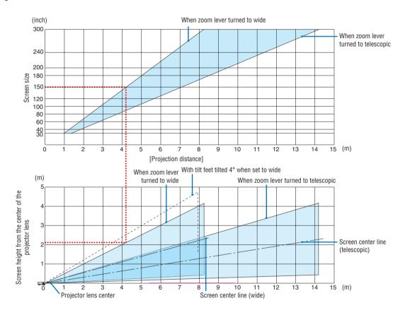
\* The figures indicated for "height of screen from projector lens center" on the projection distance table are for a lens shift of 62% V.
