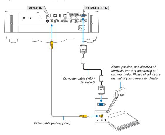
• Select the source name for its appropriate input terminal after turning on the projector.
