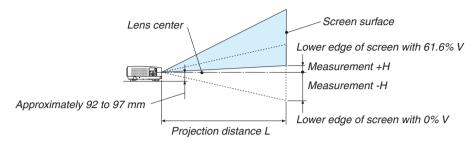
(Note) Height from lens center to lower edge of screen (with tilt feet screwed in)
