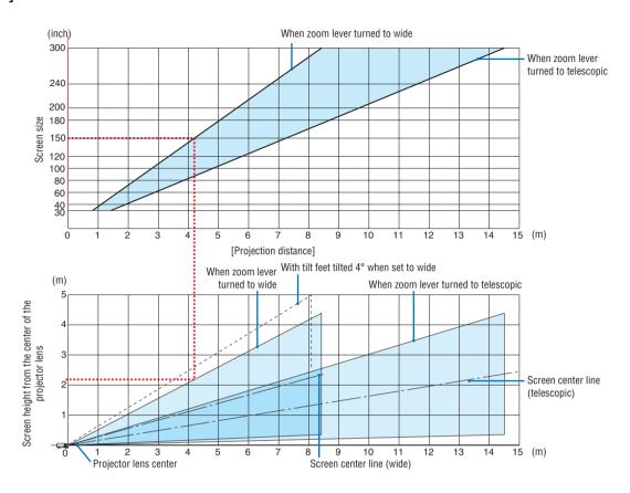
\* The figures indicated for "height of screen from projector lens center" on the projection distance table are for a lens shift of 59% V.
