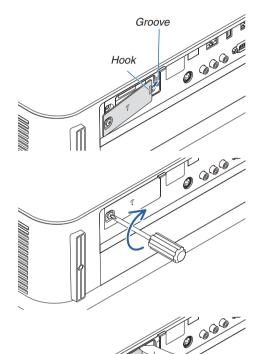
\* To remove the USB Wireless LAN Unit, disconnect the power cord and use the above procedure.
