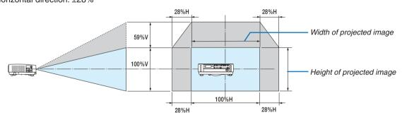
\* The lens shift range is the same for ceiling installation.
