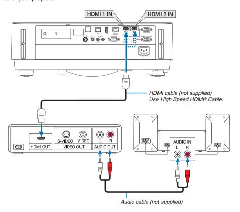
Select the source name for its appropriate input terminal after turning on the projector.
