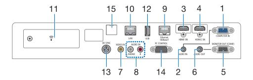
COMPUTER IN/ Component Input Terminal (Mini D-Sub 15 Pin)
