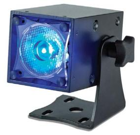
The Pica Cube can be powered via AC Mains (100-240VAC) using an available power-supply and controlled using standard DMX or in standalone mode via its easy-to-use on-board controls. The optional Pica Portal is capable of powering and controlling up to four Pica Cubes by providing power and data through a common Cat5 (24 gauge) cable.
