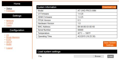
The home page will allow the user to see the general system information, download the matrix log, and save/load system settings. The information displayed will help figure out if the matrix is up to date, how long it has been running, and other key information.
