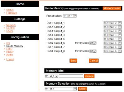
The Route Memory page provides set up, labeling, and configuration of multiple preset memories for fast and easy control.
