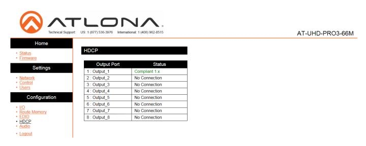
The HDCP page provides a quick way to see whether a display is HDCP compliant or not and the version supported. This page will give multiple status readouts: No Connection, Compliant 1.X, Compliant 2.X, and Non-Compliant.
