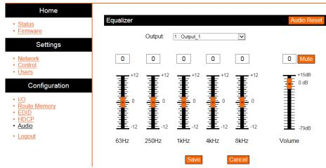
The audio page supports adjustment of 5 band EQ for the analog audio outputs ensuring the best audio performance for each zone. 5 band frequency options at 63Hz, 250Hz, 1kHz, 4kHz, and 8kHz as well as zone output volume and mute.
