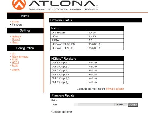
The firmware page displays the matrix, HDBaseT transmitter chips, and HDBaseT receivers firmware version and provides an easy way to update.
