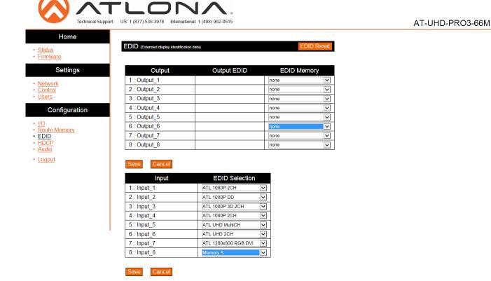
The EDID page is used for saving EDIDs, loading EDIDs, or using internal EDIDs on the input ports.
