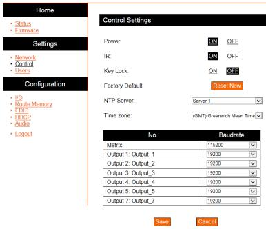
The control page will allow simple functions to be changed. Turn the matrix on/off, IR front panel receiver window on/off, and front panel key lock on/off. The time zone and baud rates (for matrix and zone outputs) can be altered as well.
