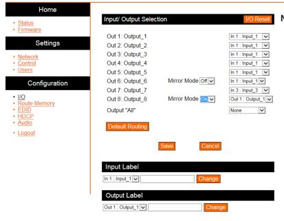
**Note:** Default label is Input\_X or Output\_X. Labels will follow corresponding ports. **Ex.** Input 6 will default to label Input\_6
