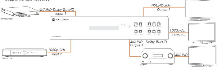
On default, all devices in the diagram will work at 1080p. If a device is not syncing or a different resolution is required, internal EDID or EDID copy and load should resolve these issues. The UHD-PRO3 can copy and store up to 8 EDIDs to memory.
