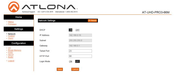
The network page enables the matrix IP settings to be altered. If a static IP is required, then DHCP needs to be turned off. Once off, the settings will be available to change.
