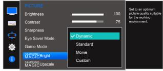
When the external input is connected through HDMI and <u>PC/AV Mode</u> is set to AV, <u>MAGICBright</u> has four automatic picture settings (<u>Dynamic</u>, <u>Standard</u>, <u>Movie</u> and <u>Custom</u>) that are preset at the factory. You can activate either <u>Dynamic</u>, <u>Standard</u>, <u>Movie</u> or <u>Custom</u>. You can select <u>Custom</u> which automatically recalls your personalized picture settings.
