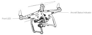
The Front LEDs show the orientation of the aircraft. The Front LEDs glow solid red when the aircraft is turned on to indicate the front (or nose) of the aircraft. The Aircraft Status Indicators communicate the system status of the flight controller. Refer to the table below for more information about the Aircraft Status Indicators:
