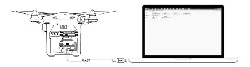
$\triangle$  The aircraft must be turned on before attempting to access the files on the Micro-SD card.
