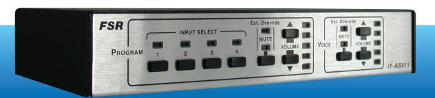
The IT-AS411 Series Audio Switchers are 4x1 audio switchers that have an extra mic/line level input for a voice lift system or direct microphone input. All models have four switched program audio inputs and an independent mic or line level input that is summed (mixed) with the selected active program audio.
