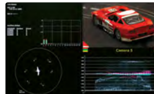
QUAD VIEWER LAYOUT Screen showing video, waveform, vectorscope, and audio levels
