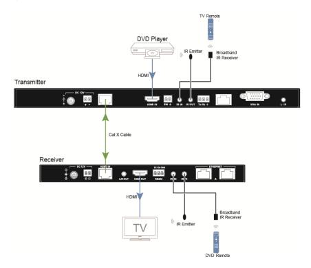
**NOTE:** It is only necessary to power one side (Tx or Rx)
