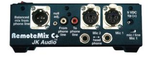
**Balanced XLR Output** delivers a line level signal containing the phone + mic mix. Adjustable to mic level with the "Line Out" control.
