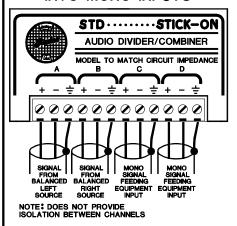
A MODULE MAY BE UNBALANCED BY CONNECTING ALL 4 NEGATIVE TERMINALS TO THE ADJACENT GROUNDS. BALANCED AND UNBALANCED WIRING MAY NOT BE MIXED.
