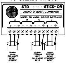
COMBINE STEREO SIGNALS INTO MONO INPUTS
