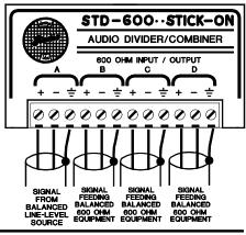
**COMBINE MULTIPLE 600** OHM SIGNALS TO SINGLE INPUT
