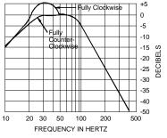
BOOST ADJUST Adjust for desired low frequency boost. This control is factory set to match the JBL Model 4645B THX approved subwoofer (THX is the registered trademark of Lucasfilm, Ltd.). This is a 25-turn control which sets the boost at 30 Hz. It may be turned counterclockwise for subwoofers not requiring this boost.
