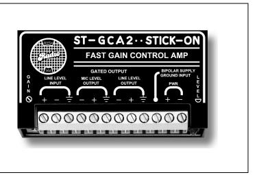
The ST-GCA1 & ST-GCA2 Gain Control Amplifiers are part of the group of STICK-ON products from Radio Design Labs. The durable adhesives provided with the ST-GCA1 and the ST-GCA2 permit permanent or removable mounting. Numerous available mounting accessories, brackets and rack-mount chassis are optionally available to facilitate any system design. The ST-GCA series products are unique, high-performance electronic modules offering constant, automatic level control of audio lines.
