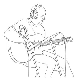
Point a small-diaphragm condenser microphone at the 12th fret, approximately 8 inches away. Point a large- diaphragm condenser microphone at the bridge of the guitar, approximately 12 inches from the guitar. Experiment with distances and microphone placement. Another popular method is using an XY microphone placement with two small-diaphragm condenser microphones. (See Drum Overheads picture.)
