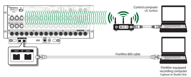
Here is a setup using wireless control by multiple devices, as would happen with band members controlling their own monitor mixes.
