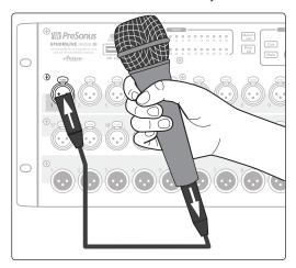
1. Plug a microphone into a mic cable and plug the cable into the StudioLive RM-series mixer's Channel 1 mic input.
