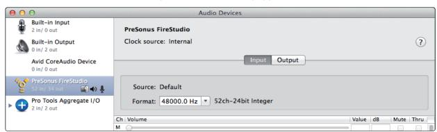
4. With Windows, the RM-series mixer uses a PreSonus FireStudio ASIO driver, installed with UC Surface, and shows up in the Sound control panel as a PreSonus FireStudio interface.
