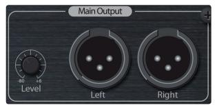
**Main Output L/R jacks:** Balanced XLR outputs carrying the left and right channel signals of the Main mix.
