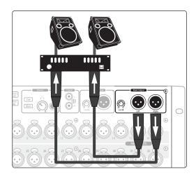
3. If you're using passive speakers, connect them to your power amplifier using speaker cables.
