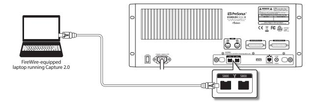
The FireWire s800 connection carries audio betwen the RM-series mixer your computer, enabling your RM-series mixer to act as a 52 x 34 FireWire recording and playback interface for Capture, Studio One, and other audio programs.
