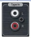
The Tape In connections on the front panel are RCA jacks that accept consumer line-level signals (-10 dBV nominal). These inputs can be used for playback from CD players, MP3 players, and other consumer devices. In UC Surface, these inputs show up as a stereo tape return channel strip. For more information, see Chapter 4, "UC Surface," in the StudioLive-Al Software Library Manual.
