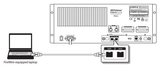
A single computer can be used both to control and to record from the RM-series mixer, or separate computers can be used for control and audio.
