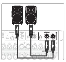
2. Connect the Main Outputs of your RM-series mixer to your power amplifier or powered monitors.
