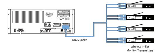
Balanced DB25 fan-out snakes (breakout cables) can be obtained in various configurations at most recording and live-sound retailers. Common fanout configurations are DB25-to-(8) XLR-M and DB25-to-(8) ¼-inch TRS.
