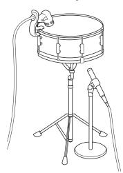
Point a dynamic microphone at the center of the snare, making sure it is placed so that the drummer will not hit it. Place a small-diaphragm condenser microphone under the drum, pointed at the snares. Experiment with the placement of both microphones. Also experiment with inverting the polarity of the bottom microphone. This technique can be used in live applications.
