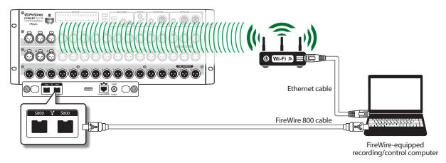
4. Separate computers for control and audio, with both connections wired.
