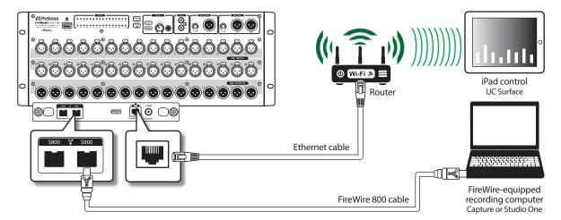
Separate computers for control and audio, with the RM mixer connected wirelessly to the router.
