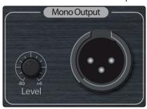
The XLR jacks are electrically balanced and rated +24 dBu maximum output level. They are wired as follows:
