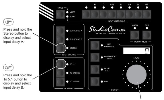
Use the level control to adjust the input delay. Range is from 0 to 340. The display shows delay in milliseconds at 48 kHz sampling rate. The value is scaled up or down for other sample rates.
