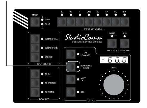
**Default:** Reference level set for –60.0 dB post-fader monitor output level.
