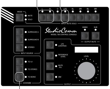
Press and hold the To Mono button to display and confirm the LFE downmix level and pre-fader monitor output mode.
