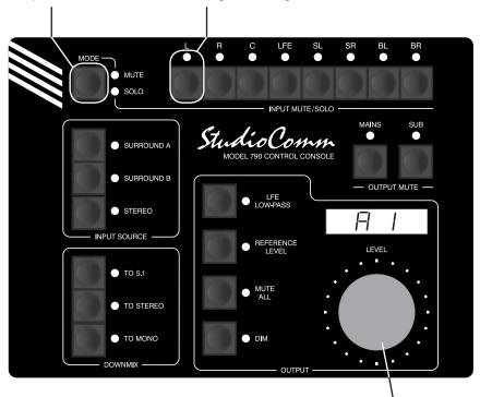
Use the Level control to change this specific Model 790's device address. Address can be either A1, A2, A3, or A4. See Note below.
