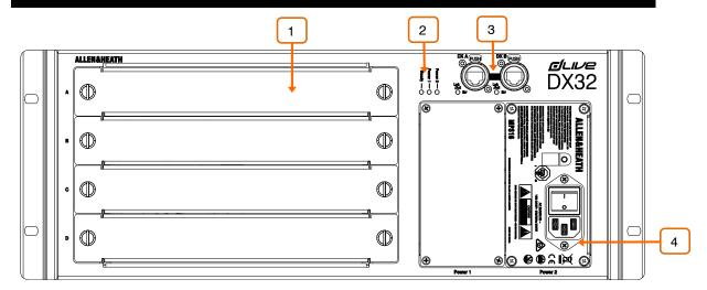
1 I/O modules – 4x slots for fitting 8ch analogue or digital I/O modules. To fit a module, switch the expander off, remove the blank panel by loosening the 2 thumb screws, slide the module into the slot and press it firmly into the mating connector, then secure it by tightening the thumb screws.
