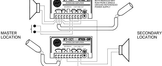
INTERCOM USING SEPARATE MICS AND SPEAKERS
