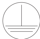
Figure Protective Conductor Terminal Symbol
