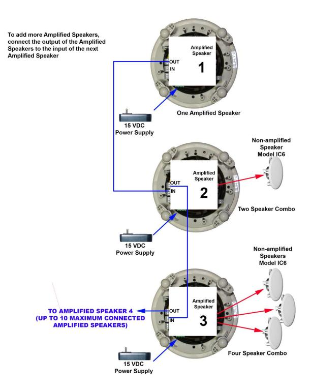
**Chained Self Amplified Speakers Wiring**
