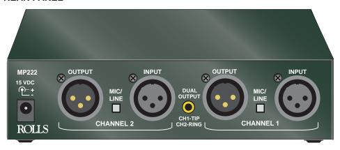
INPUTS: 1 - 2: XLR balanced inputs for connection to any standard dynamic or condenser microphone. The input circuitry has a very wide input range and can accommodate almost any (mic to line) level signal if you select the proper setting for the Mic/Line switch.
