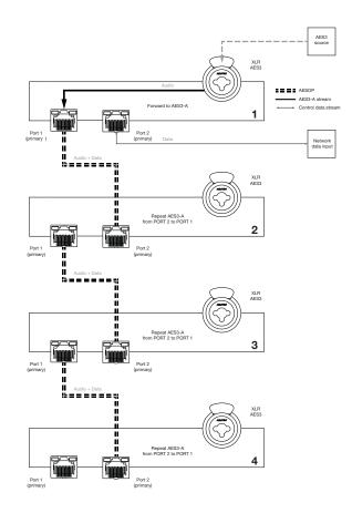
FIGURE 41: Daisy chain - two port models.
