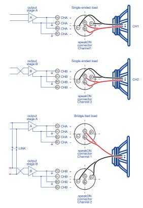
FIGURE 12: Loudspeaker connections: singleended loads (top), bridged-tied load (bottom).
