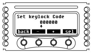
FIGURE 51: Setup: Set the keylock code.
