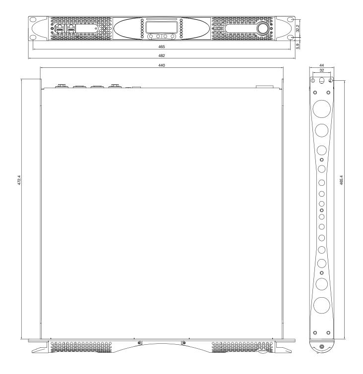
FIGURE 3: K6, K8, K10 and K20 mechanical drawings.
