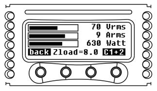
FIGURE 47: Display: Output meters.
