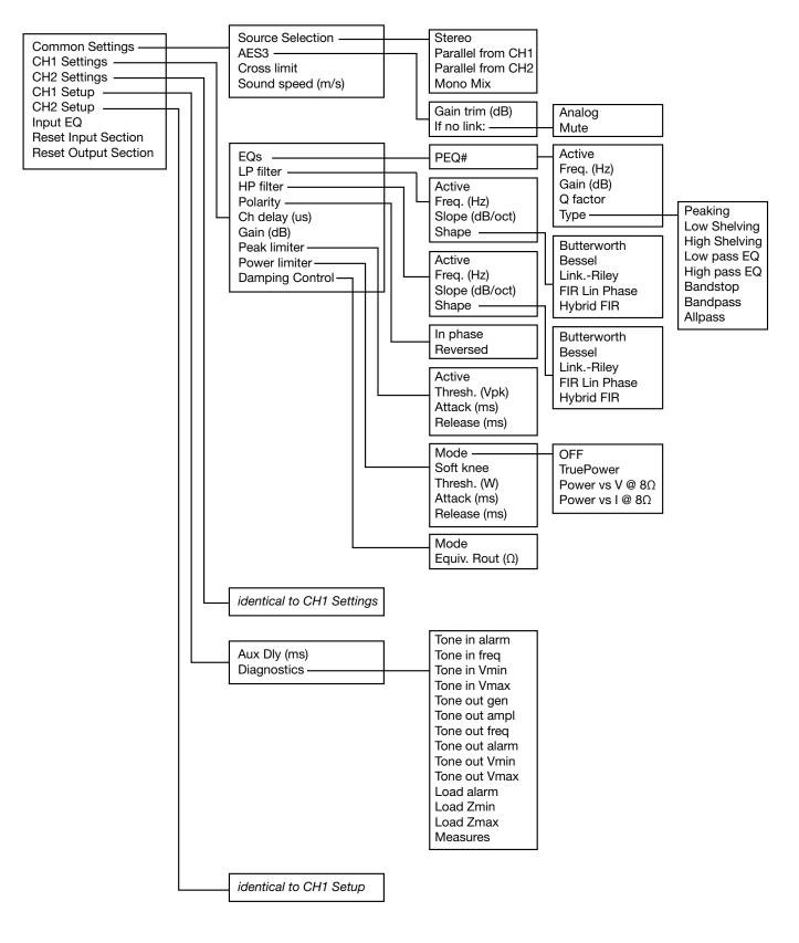
FIGURE 21: DSP settings diagram.
