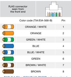
TABLE 1: EtherCON/RJ45 T568B scheme pinout.
