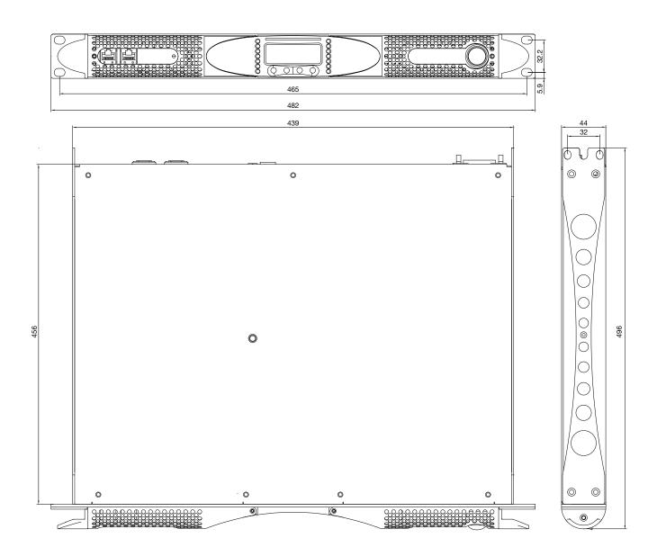
FIGURE 2: K2 and K3 mechanical drawings.
