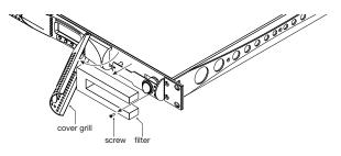
FIGURE 6: Cleaning air filters.
