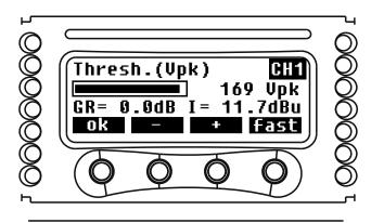
FIGURE 31: Peak limiter: threshold voltage and gain reduction.
