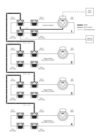
FIGURE 40: Daisy chain - four port models.
