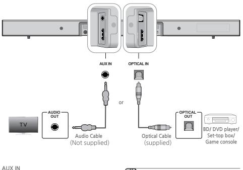
Connect **AUX IN** (Audio) on the main unit to the AUDIO OUT jack of the TV or Source Device. Change the function to **AUX**.
