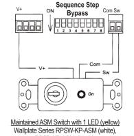
RPSB-KP-ASM (black), Alternate Sequence Mode (ASM) allows for the
