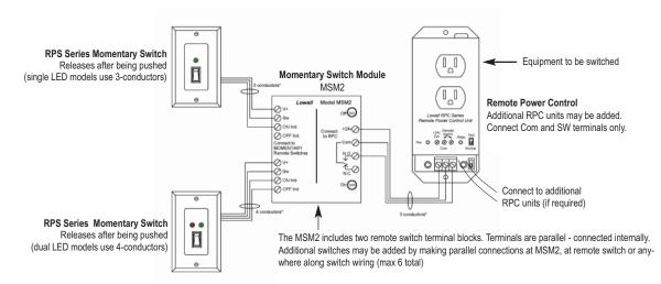
Wiring Notes: Maximum distance between switches, MSM2 and RPC is: 22 ga: Max distance is 6,600 ft. (1.25 miles), 18 ga: Max distance is 17,160 ft. (3.25 miles)
