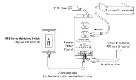
Wiring Notes: Maximum distance between switch and RPC is: 22 ga: Max distance is 6,600 ft. (1.25 miles), 18 ga: Max distance is 17,160 ft. (3.25 miles)
