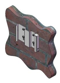
Slide the mating Mounting Bracket (attached to the Unit) into the Mounting Bracket Base until the locking clip engages, and install the provided 8-18 x .500" SS Thread Forming Torx Button Head Security Screw, in the hole on the left side of the Bracket assembly.
