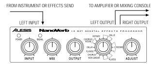
Stereo. Connect two 1/4" phone cords to the [LEFT] and [RIGHT] INPUTS of the NanoVerb from a stereo source, and two other 1/4" phone cords from the [LEFT] and [RIGHT] OUTPUTS of the NanoVerb to a stereo amplification system or two mixer inputs.
