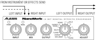
If connecting to a mixing console's aux sends/returns, you will want to turn the [MIX] knob fully clockwise so that the NanoVerb outputs only wet (effected) signal.
