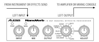
Mono In, Stereo Out. While still using a mono input, you could connect two 1/4" phone cords to the [LEFT] and [RIGHT] outputs of the NanoVerb to a stereo amplification system or two mixer inputs.
