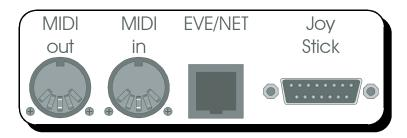
At the back of the remote are four connectors, as shown above. Only the EVE/NET connector is required to be connected, the use of rest is optional.
