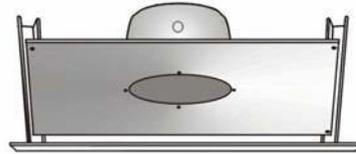
3. After hole is cut in the ceiling, connect the wires and install the speaker by tightening the screws of the four clamps.
