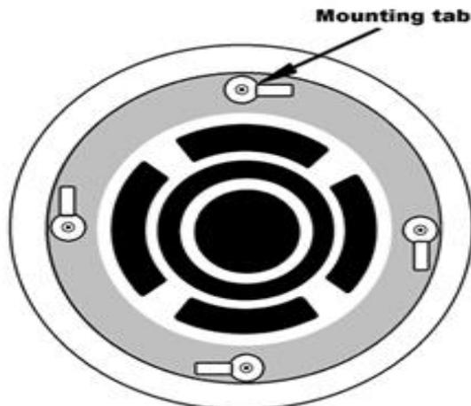
Be sure to position the four Mounting Tabs on your OWI speaker inward then insert the four (4) screws (supplied) from the front of the speaker into the screw opening.
