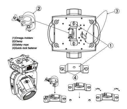
Screw one clamp each via a M12 screw and nut onto the Omega holders. Insert the quick-lock fasteners of the first Omega holder into the respective holes on the bottom of the Vizi Beam Hybrid 2R. Tighten the quick-lock fasteners fully clockwise. Install the second Omega holder. Pull the safety-cable through the holes on the bottom of the base and over the trussing system or a safe fixation spot. Insert the end in the carabine and tighten the safety screw.
