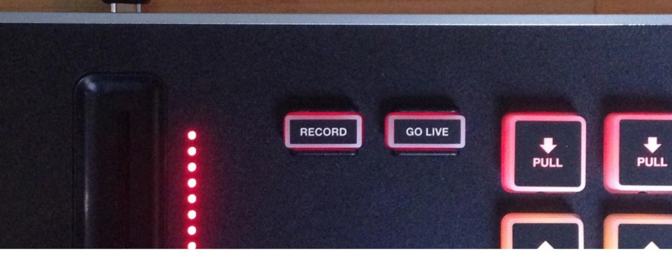
Finally, the Surface Go includes buttons that allow you to start and stop your recordings and streams.
