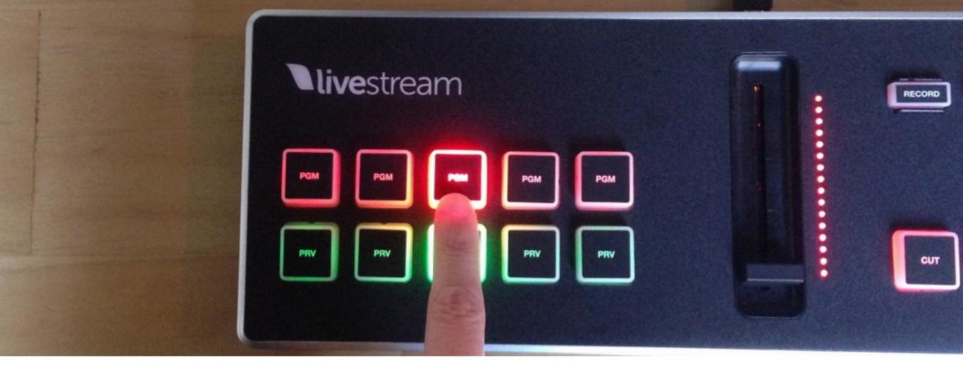
Similarly, to put a source directly into Program, press the corresponding 'PGM' button.
