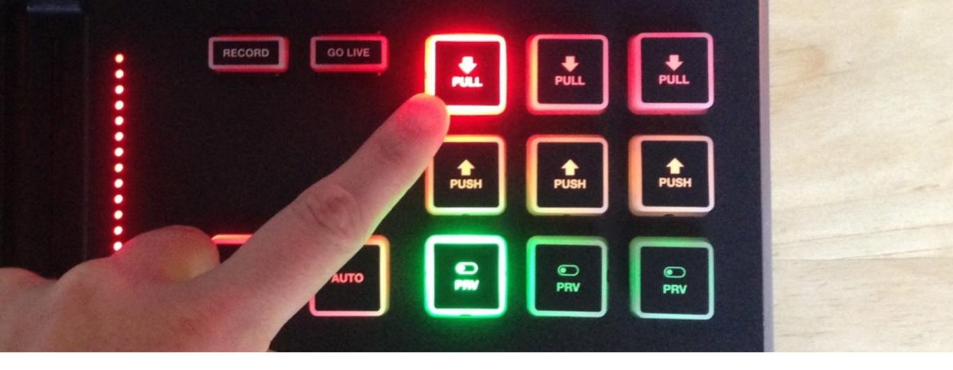
The red 'PULL' button will light up, indicating that the graphics overlay is in Program. Press it to remove the graphic from Program.
