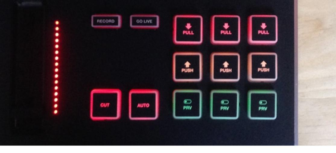
The right side of the Surface Go features the graphics overlay controls for all three graphics channels.
