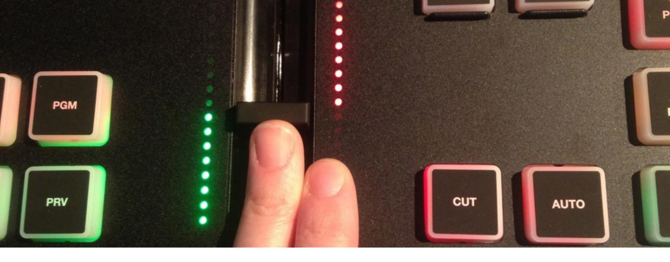
The Surface Go also includes a mini T bar to execute a manual transition, allowing you to control the speed of a dissolve or wipe.
