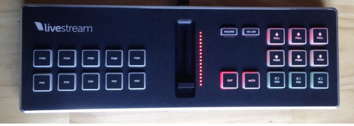
Launch Livestream Studio, or relaunch if it is already open. Some of the buttons on the Surface Go will light up slightly when the software has finished launching.
