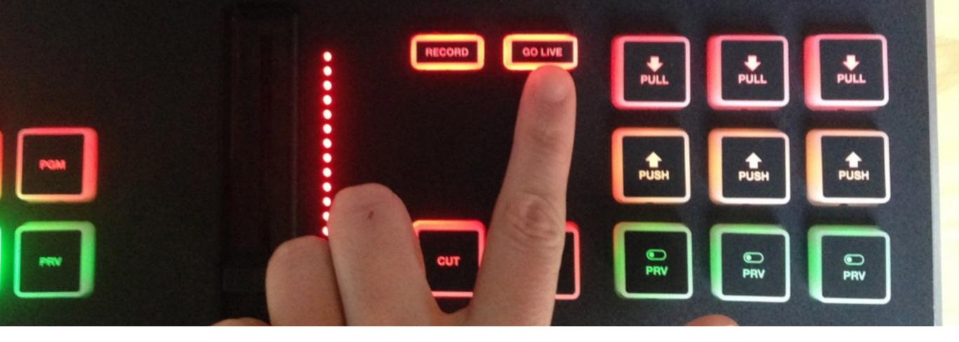
When you first press either button, they will light up red to indicate that they are active. Press the button again to stop the recording or streaming.
