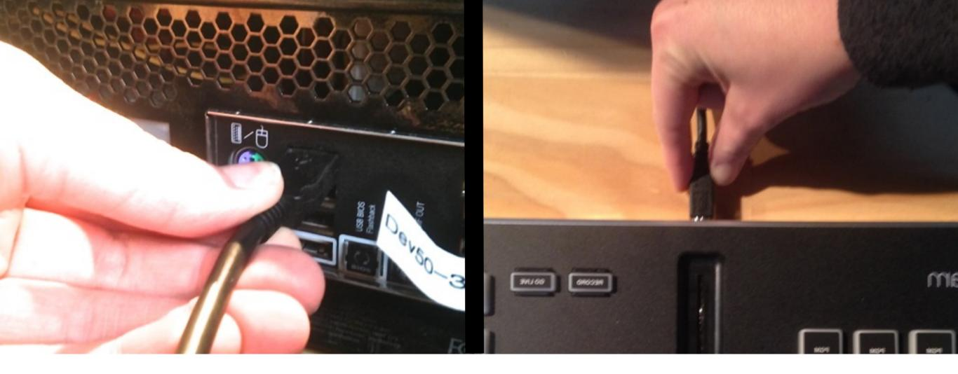
Start by connecting the USB cable to the Surface Go and plugging it into a USB 2.0 port on your Livestream Studio system. The drivers will install automatically.
