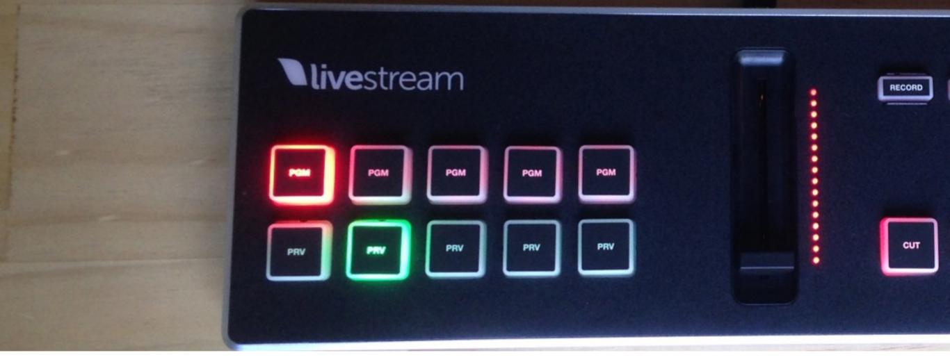
After saving your settings, the Surface Go will indicate which of your assigned sources are in Preview and Program. The track with the lit green 'PRV' button is in Preview. The track that has the lit red 'PGM' button is in Program.
