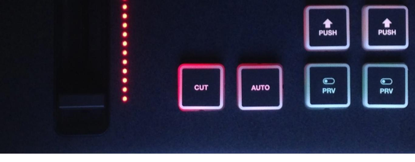
The Surface Go also includes 'Cut' and 'Auto' transition controls for switching sources between Preview and Program.
