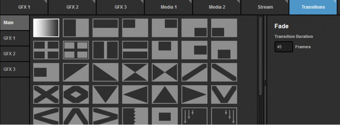
The 'Auto' transition type and speed is determined in Livestream Studio under the '**Transitions**' tab.
