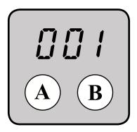
The control panel LED display shows the menu items you select from the menu map on page #11. Press the **<A>** button repeatedly until you reach the desired menu function. When a menu function is selected, the display will immediately show the first available option for this selected menu function.
