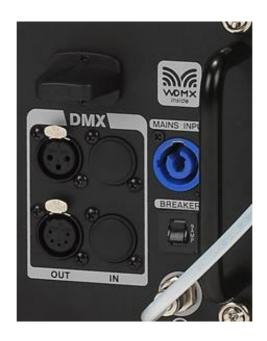
Address Setup – Use control menu to set DMX address. The machine occupies 2 control channels. The starting address is defined as the first channel from which the machine will respond to the controller. Always double check to make sure there are no overlapping channles in order to control the machine correctly.
