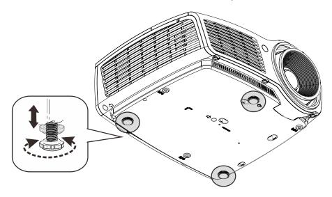
To adjust the angle of the picture, turn the tilt-adjuster right or left until the desired angle has been achieved.
