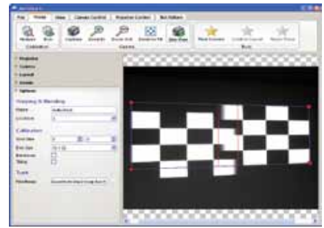
▲ The user interface guide directs you step by step through the set-up process including: projector selection, screen corner detection, blend region percentage and all the way to the final blended and/or stacked image.
