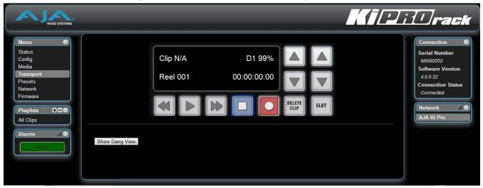
STOP : Press STOP to end playback or a media operation (PLAY, FF, REV, or RECORD). When stopped, Ki Pro Rack displays the current point in the stopped clip. STOP can also be considered a "pause" button. A double-press of the STOP button will return Ki Pro Rack to an E-to-E state.
