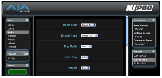
Media State (12.1): This parameter defines whether the media is used for video/audio recording or data transfer using an Ethernet LAN.
