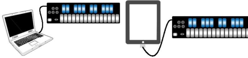
QuNexus is connected and powered using the Micro USB port on the left side of the QuNexus. It is a class compliant USB device and does not require a driver. This allows for maximum compatibility with an extremely wide range of other devices.
