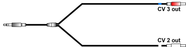
3.5mm (1/8in) stereo plug to dual 3.5mm (1/8in) mono plugs
