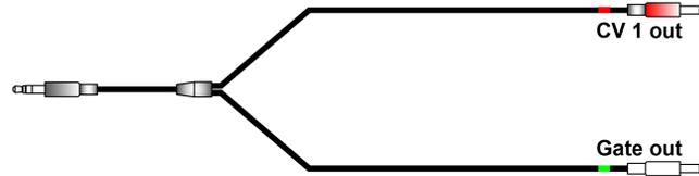
3.5mm (1/8in) stereo plug to dual 3.5mm (1/8in) mono plugs
