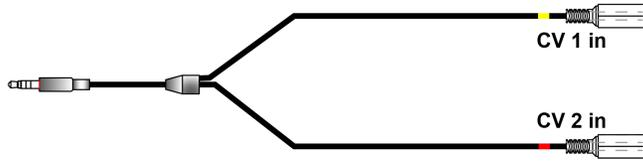
3.5mm (1/8in) TRRS plug to dual 3.5mm (1/8in) stereo jacks
