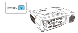
**Note:** To shut down the projector, press the  $\bigcirc$  power button twice, then unplug it. You don't have to wait for the projector to cool down.
