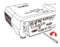
Connect the wireless LAN module to the USB-A (flat) port.
