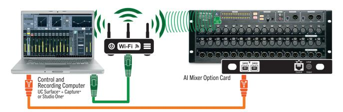
Ethernet Control + FireWire Recording
