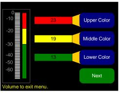
Upper Segment: Pressing this button and then rotating the Channel Volume knob adjusts the division between the upper and middle segments. You can adjust the color boundary in one dBr increments, and it has the same range as the bottom and top limits of the meter.
