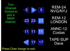
Basic instructions are on the screen. Press the **Channel Select** button corresponding to the metering channel position you want to reassign. It will highlight in yellow.
