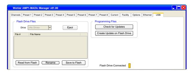
The **Flash Drive Connected** indicator (bottom right of the screen) shows when a flash drive is connected to the USB port of the host computer by turning gold (on). Otherwise, it is brown (off).
