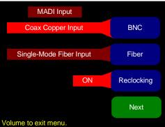
3. Press either **BNC** or **Fiber**. This menu contains a variety of useful options that can be used to customize the AMP1-MADIe to your needs. Refer to Chapter 4 for details. Exit this menu by pressing **Next** or pressing the **Channel Volume** knob for at least three seconds.
