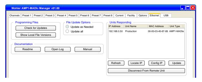
The **Ethernet** tab allows you to transmit configurations and perform a variety of other tasks over a network. It also allows you to connect to an AMP1-MADI*e* over a LAN to remotely configure the unit.
