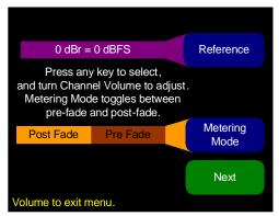
Press the **Metering Mode** button to change between **Post Fade** and **Pre Fade**. Then press the **Back** or **Next** buttons several times to exit to the **Main Screen**.
