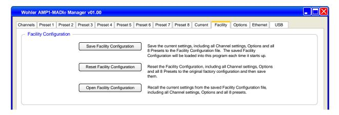
You can access the **Facility** tab whether an AMP1-MADIe is connected or not. It is a complete AMP1-MADIe configuration, including all channel settings, all presets, and all options and intended to contain the basic settings that are typically needed facility-wide. You can only have one facility configuration file at a time.
