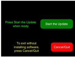
Pressing **Start the Update** button will start the installation process, which will automatically continue until its conclusion. Instructions are provided on this screen to explain the process. When the software is finished installing, the AMP1-MADIe will restart and the **Main Screen** will display.
