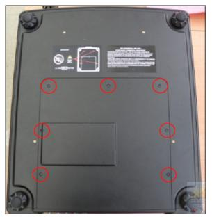
3. Remove and retain the 13 screws securing the main board upper shield. Remove the shield.
