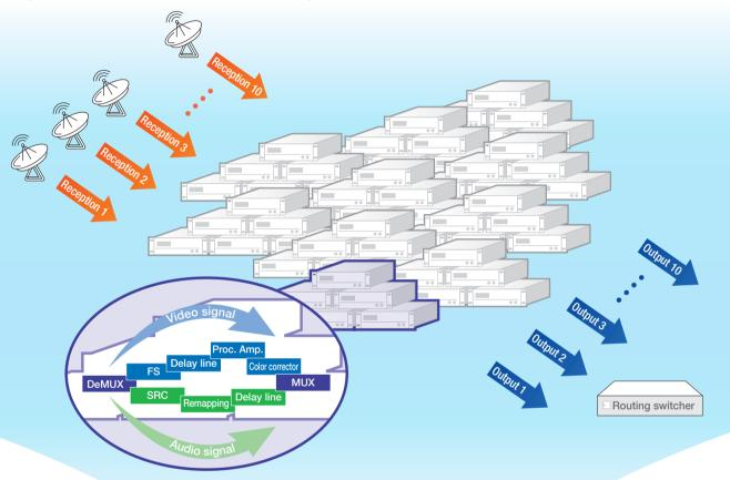
Integrates various signal processing units that required separate equipment for each channel into a single FA-1010 unit
