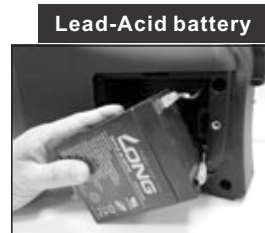
Remove connectors and replace new battery in reverse order RED = Positive; BLACK = Negative
