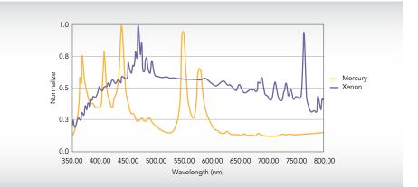
A Xenon vs high pressure Mercury lamps
