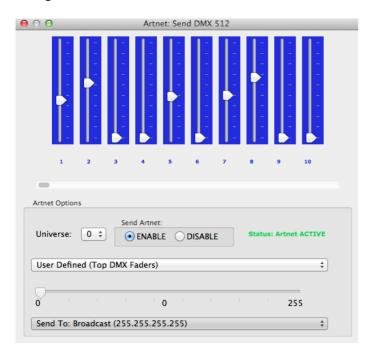
When first opened, the Art-Net is set to Disabled, please set it to Enabled, and then you can use either the DMX faders to test one or more DMX channels, or use the testpatterns from the options available.Set the universe to be the same as configured on the ODE, and change the Send to either broadcast or send direct to the ODE IP address
