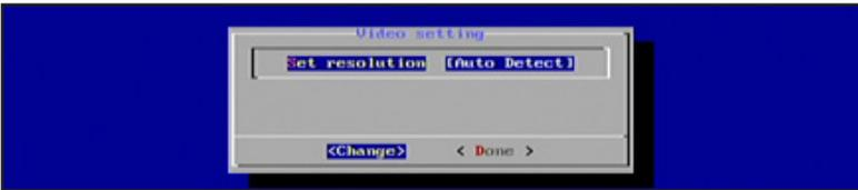
2. The Video Setting dialog will display the current resolution. Press the Enter key once again to display a list of the available output resolutions.
