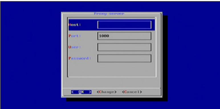
3. Use the Change option to modify the information in each field. After each field has been filled with the proper information, highlight OK and press the Enter key.
