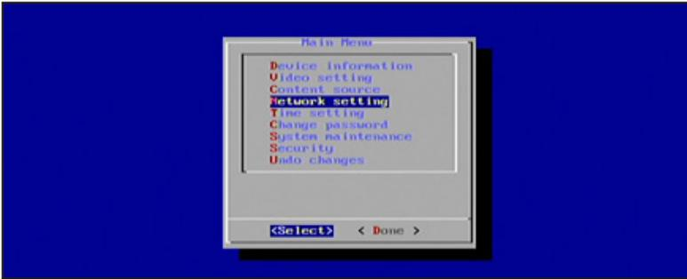
2. Press the Enter key to display the Network Setting dialog. The IP Configuration option is selected by default.
