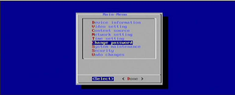
2. Enter the password under the Change Password dialog. If no password was previously set (or if the unit has been reset), then the Old Password field will be blank. Use the ▲ and ▼ keys to move between each field.
