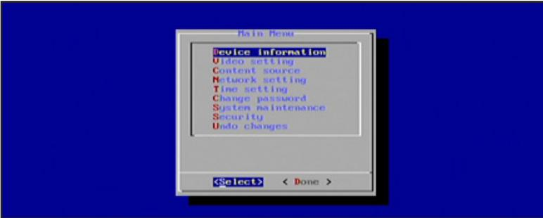
Once the Main Menu is displayed, use the Arrow (cursor) keys, Spacebar, Enter Key, and Numeric Keypad to navigate the Main Menu. Use the Arrow (Cursor) Keys to highlight a menu item. Press the Spacebar to make the selection by placing an asterisk (\*) next to the highlighted item. Press the Enter key to confirm the selection.
